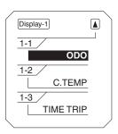
5. Repeat the previous step to make other item changes, or if you are finished adjusting the information display page items, use the select switch to highlight "a", and then push the menu switch "MENU" to exit.
