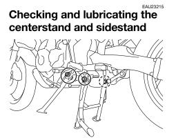
The operation of the centerstand and sidestand should be checked before each ride, and the pivots and metal-tometal contact surfaces should be lubricated if necessary.
