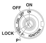
The main switch/steering lock controls the ignition and lighting systems, and is used to lock the steering. The various positions are described below.
