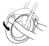
The front and rear wheel bearings must be checked at the intervals specified in the periodic maintenance and lubrication chart. If there is play in the wheel hub or if the wheel does not turn smoothly, have a Yamaha dealer check the wheel bearings. Battery
