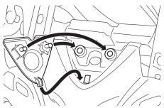
14. Install the windshield by installing the screws, and then tightening them to the specified torque. WARNING! A loose windshield
