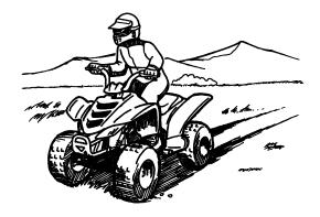
If the rear wheels of your ATV start to slide sideways, control can usually be regained (if there is room to do so) by steering in the direction of the slide. Applying the brakes or accelerating is not recommended until you have corrected the slide.
