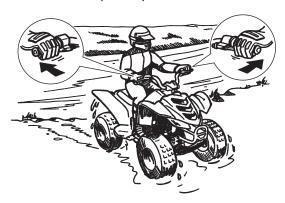
After riding your ATV in water, be sure to drain the trapped water by removing the check hose at the bottom of the air filter case. *NOTICE:* Undrained water can cause damage or improper operation. [ECB00842]
