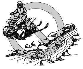
Test your brakes after leaving the water. If necessary, apply them several times to let friction dry out the linings. Do not continue to ride your ATV without verifying that you have regained proper
