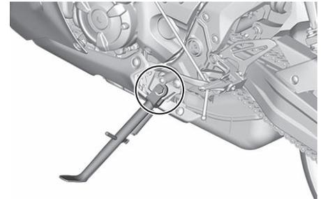
The operation of the sidestand should be checked before each ride, and the sidestand pivot and metal-to-metal contact surfaces should be lubricated if necessary.
