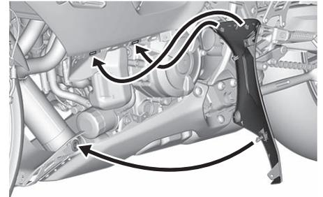
3. Install the bolts, washers and the quick fastener screws.
